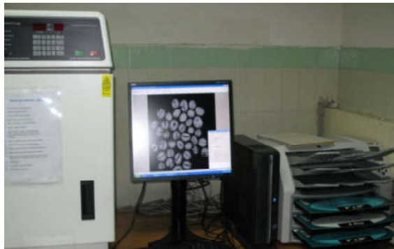
Fig.1. Faxitron SR MX 200 real-time X-ray machine for detection of hidden infestation of bruchids in seeds. The seeds are spread in a small plastic tray and exposed to soft X-rays generated at 19-26 kv. For 19-25 second depending on the seed size using the real time X-ray machine, Model No. Faxitron SR MX-200. As the machine is real-time, it automatically gives the X-ray radiograph on the monitor (Fig.2).
