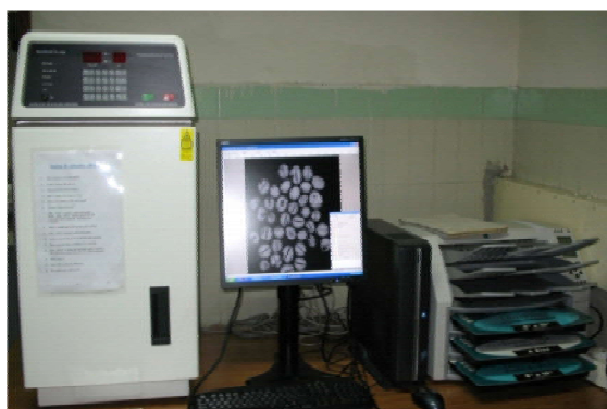
Fig.1 Faxitron SR MX 200 real-time X-ray machine for detection of hidden infestation of bruchids in seeds. The seeds are spread in a small plastic tray and exposed to soft X-rays generated at 19-26 kv. For 19-25 second depending on the seed size using the real time X-ray machine, Model No. Faxitron SR MX-200. As the machine is real-time, it automatically gives the X-ray radiograph on the monitor (Fig.2).
